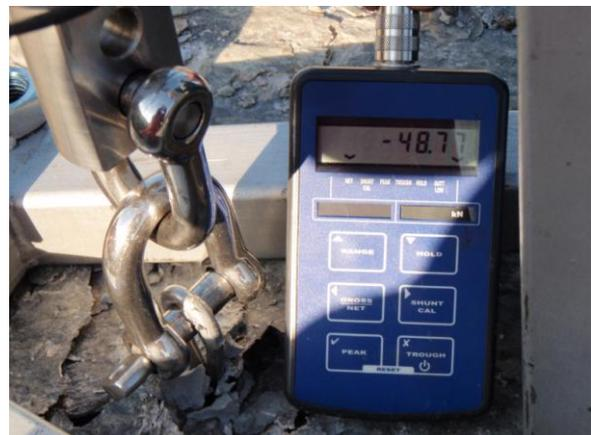
Another interesting observation was that the shank of the Bolt Products anchor unwound and elongated under loads approaching 50kN. (5<sup>th</sup> anchor from right picture below). The deformation loads were similar to the previous test. The ultimate failure load i.e. the peak load at which the anchor started to egress from the resin or the load required to extract the anchor from the resin, or substrate failure, whichever was higher, was within the range 32 - 63kN with a mean of 44.91kN.
